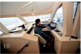
top level equipment and running rigging, this is an extremely safe position, highly workable and ergonomically perfect. You're not running from right to left, and everything is controlled from a central console served by two powerful Harken electric winches. This organization and the resulting freeing up of space for access across the coachroof will allow a couple to manage this big boat easily over long distances.
